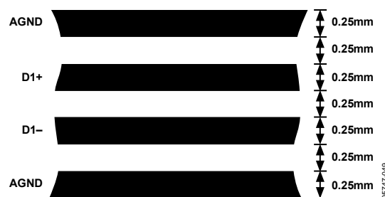
Figure 61. Arrangement of Signal Tracks
